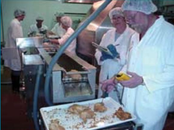
*TAKING MEASUREMENTS - John Marcy, far right, takes measurements on chicken breasts to ensure proper cooking temperature.*
