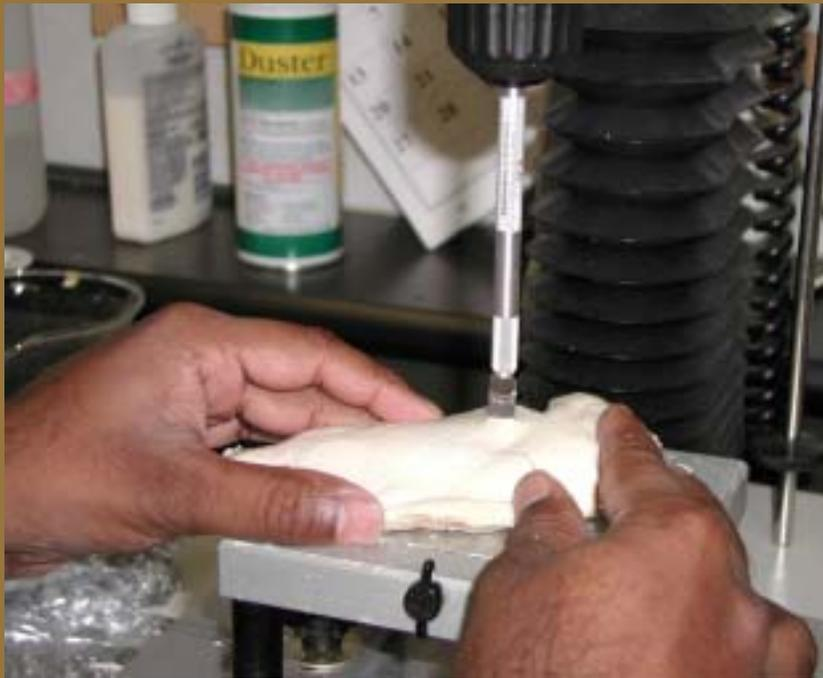
*SHEAR PRECISION - A researcher is shown evaluating tenderness by using the razor blade method to shear through cooked broiler breast meat. This method has been superior in predicting poultry meat tenderness and has less sample preparation involved, making it more efficient than other methods of prediction.*
