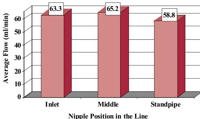
**Figure 5. Average Nipple Water Flow in House 1 of the UA Broiler Unit - Middle Up**
