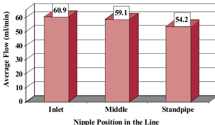
**Figure 4. Average Nipple Water Flow in House 1 of the UA Broiler Unit - Inlet Up**
